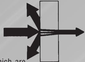
**3. DAMPING:** Materials which are vibrating are sometimes re-radiating this energy as sound by driving the air adjacent to their surface. Damping materials are applied directly to the vibrating surface and convert this energy directly into heat via minute deflections.
