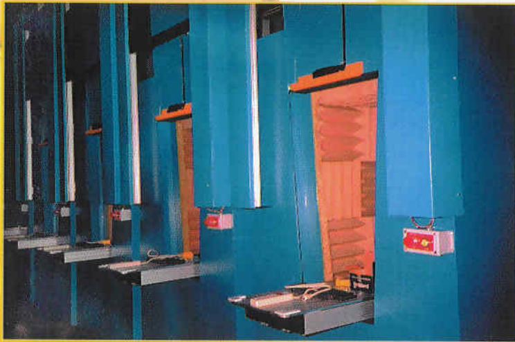
PLC Controlled Acoustic Test Chambers Automate Sound Level Testing
