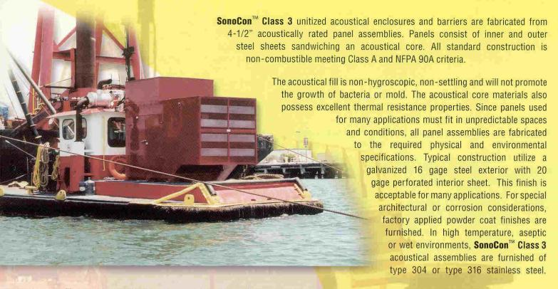
SonoCon™ Class 3 acoustical panels provide both significant sound transmission loss performance and sound absorption characteristics.
