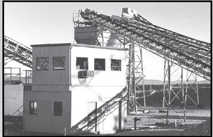
Personnel and equipment within the control rooms are isolated from high temperatures, dirt and noise. The building is self-contained, complete with emergency power systems, housing the computerized operating system at this automated cement batch plant.
